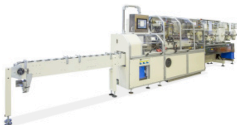
The SW 700-D is managing products with different sizes and shapes, and several wrapping materials Source: Acma
