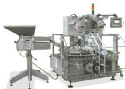
The HW 900 is a fold wrapper for high-speed double twist round candies Source: Acma
