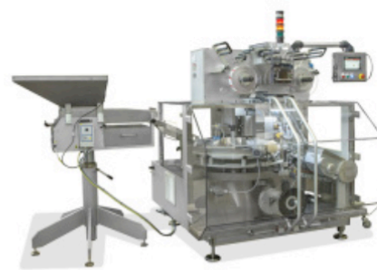
HW 900 is said to boast top performance with a packaging speed of up to 900 pieces/minute Source: ACMA
