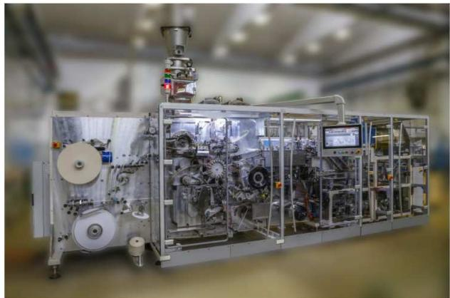
But the characteristics that made it a unique solution in the entire market remain unchanged: the capability of manufacturing double chamber type bags without using glue or staples, with the knotted tag arranged on the front package side, resulting in pleasant appearance and friendly usability.
